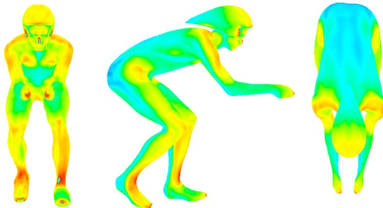
Figure 1. CHTC distribution on the cyclist's surface for different positions for  $U_\infty = 60$  km/h, made dimensionless with the surface-averaged CHTC of the cyclist ( $CHTC_{cyclist}$ ), for front view, side view and top view.
