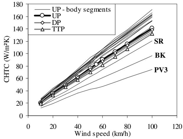
**Figure 8.** Correlations of CHTC with the wind speed ( $U_\infty$ ) for the cyclist (for UP, DP and TTP) and for the individual body segments (only for UP). The body segments which show a low CHTC are indicated (PV3: pelvis3, BK: back, SR: side right).
