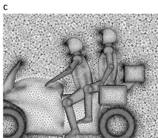
Figure 6. Computational grid in vertical center plane and on body of cyclist and motorcycle.
